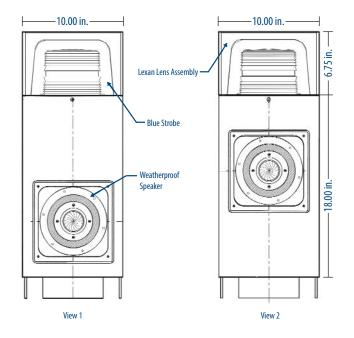
Each Model 234SBM Stanchion Broadcast Module is shipped in kit form for field installation. Components included with each complete stanchion module are as listed below.
